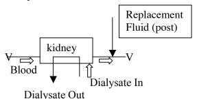
\*To prevent hemoconcentration and clotting of the blood as it goes through the hemofilter, replacement fluid is usually infused prior to the hemofilter (pre-filter) rather than after it (post-filter).
